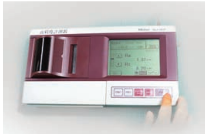
SURFACE ROUGHNESS TESTER
